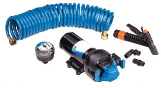
Robust five chamber, patented co-injected molded diaphragm and larger heavy-duty motor brushes significantly extend pump life by up to 50%. The HotShot Series Washdown Pumps are available in 4.0 GPM (15.1 LPM), 5.0 GPM (18.9 LPM) and 6.0 GPM (22.7 LPM) with pressures up to 70 psi (4.8 bar) and are self-priming up to 10¹ (3m).
